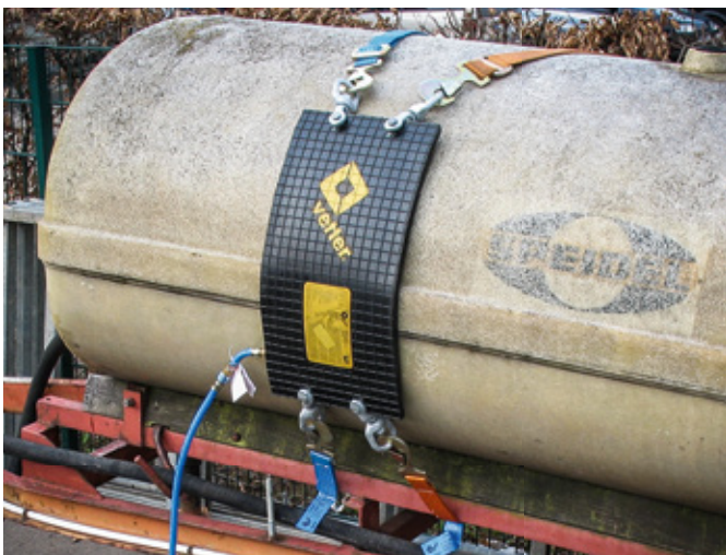
leak sealing bags with swivel eyes
