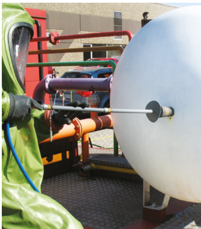
Seal leaks from a safe distance
